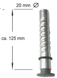
Perm. Load at application of Mortar Grout "POWER STAR" at  $5^{\circ}$  C min.:  $F_h$  40 kN after 3,0 h. mature time with concrete property 25 N/mm<sup>2</sup> Care for Application Instruction!
